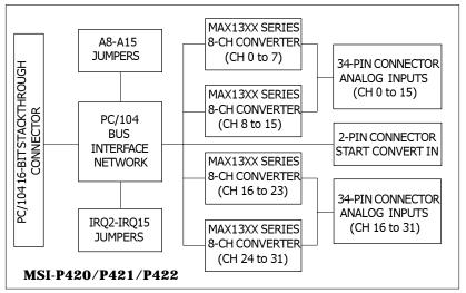
Figure 1. Block Diagram of the MSI-P420/P421/P422.
