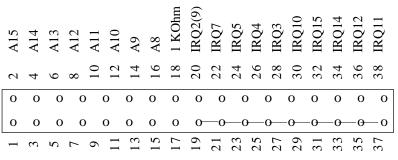
Figure 3. Jumper block JP1 configuration.
